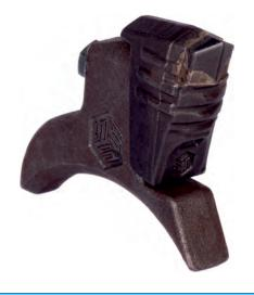
The tool MONO is used in Rotovator for harder material. The large and massive carbide part of this tool crushes harder material at high penetration force and with a long service life.
