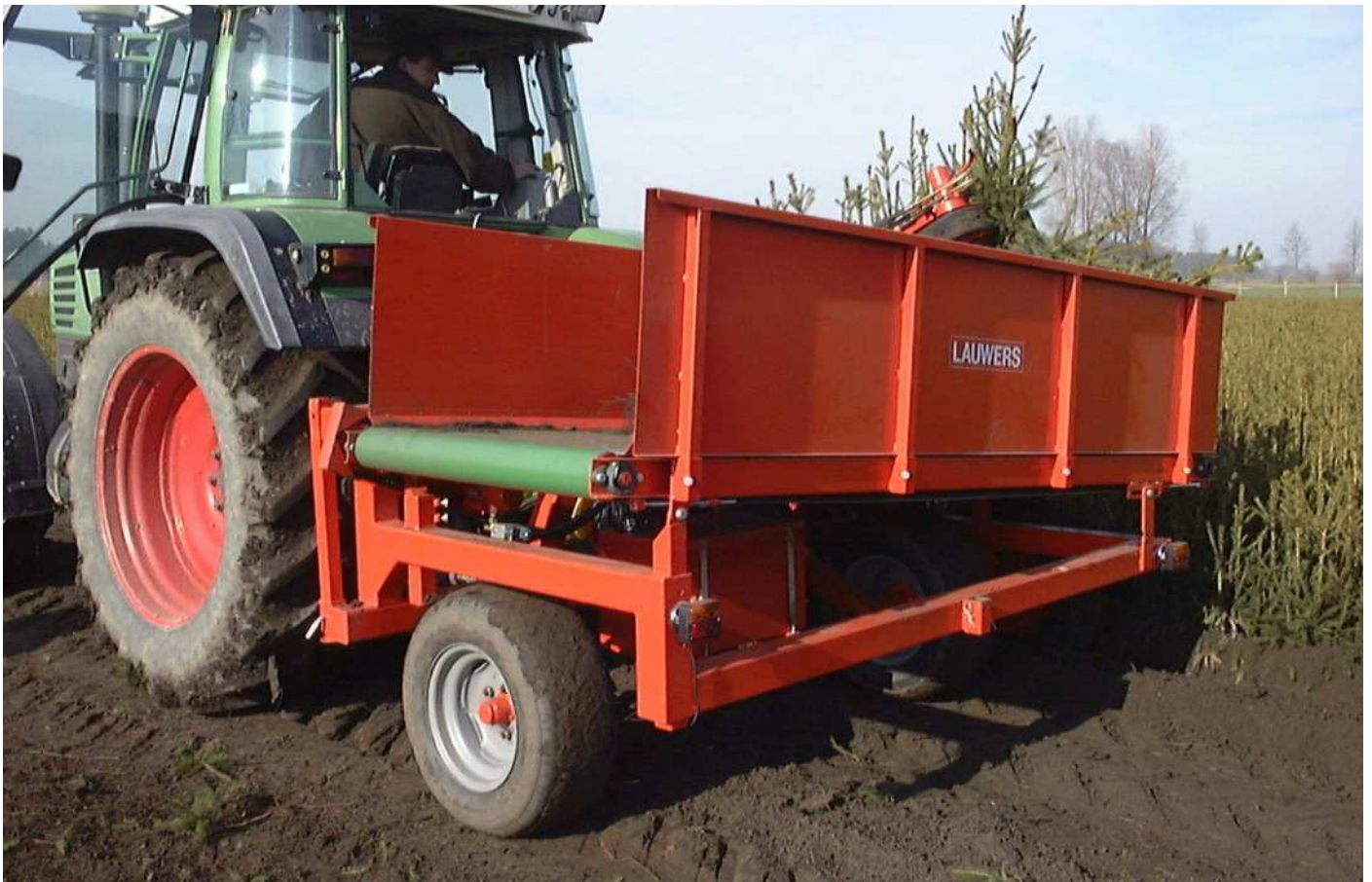
custom made machine with bunker for small christmas trees
