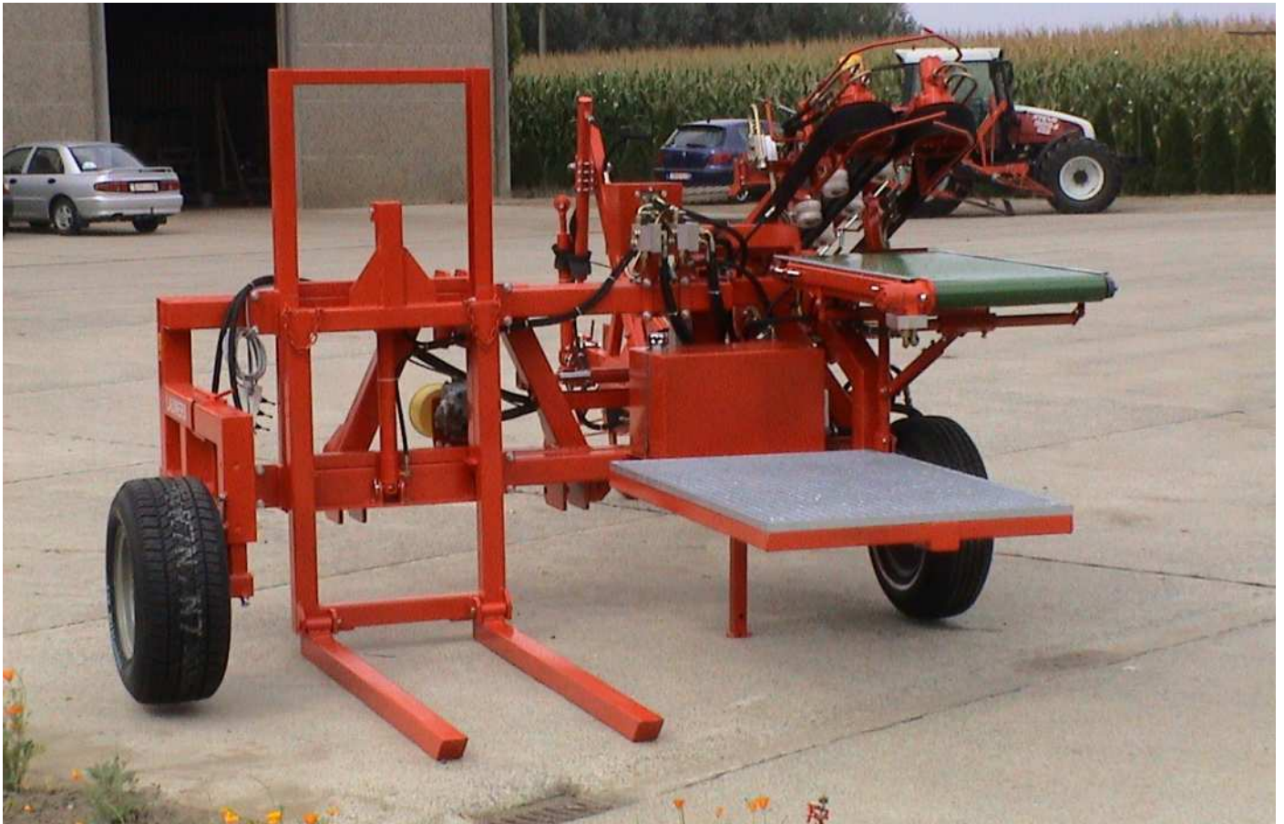
ZL, left wheel can be twisted to reduce the width of the machine on the road
