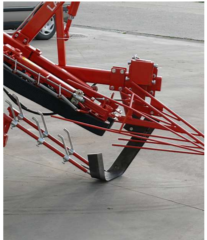
Lifting blade and shaker (the same for all models)
