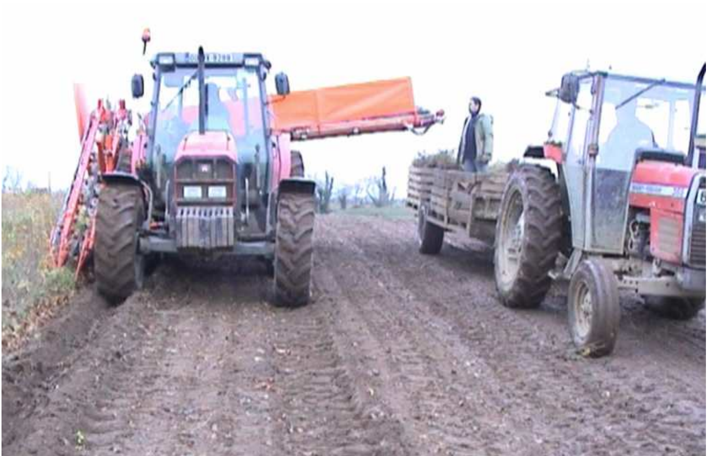
custom made machine to load directly on a trailer
