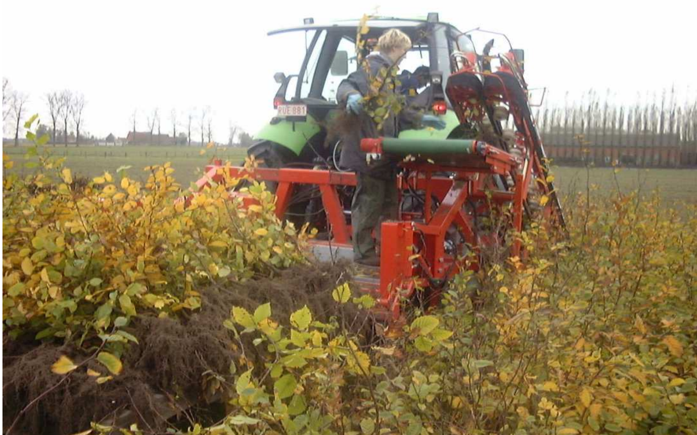
AL, with standard conveyor belt 1 m long, can be turned to the side or to the back
