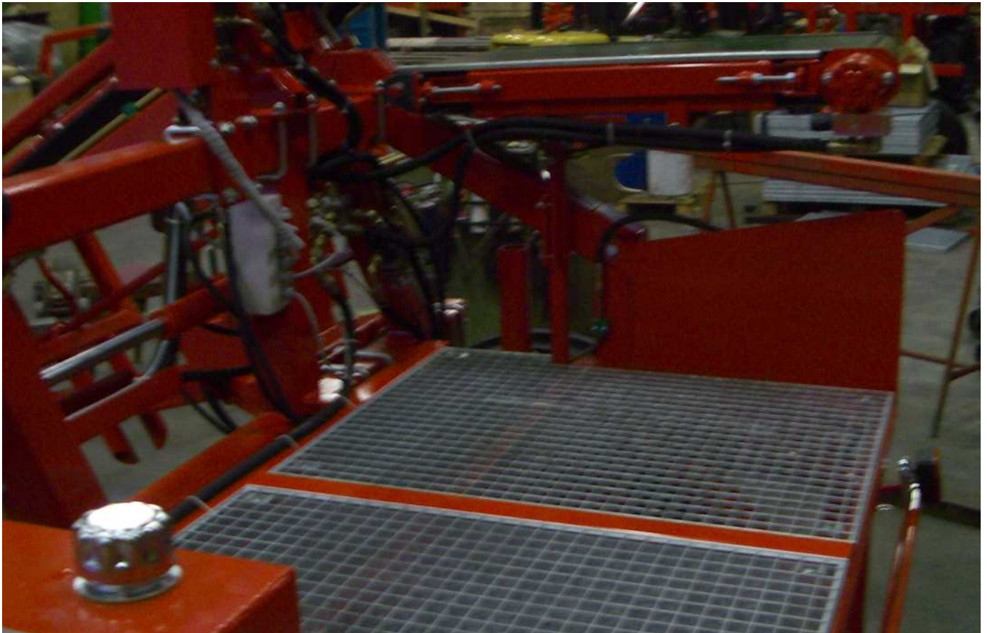
ALC, almost the same frame as AL, but shorter = weight of pallet closer to the tractor. Elevator on the back with 2 or 4 forks.
