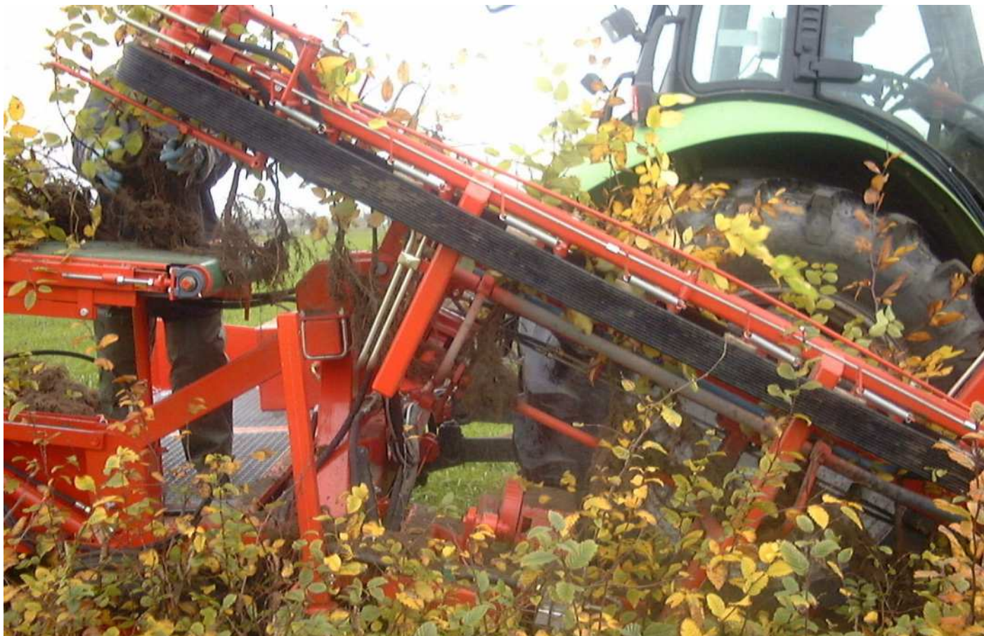
AL : elevator at the back with 2 or 4 forks, platform 1,3m long
