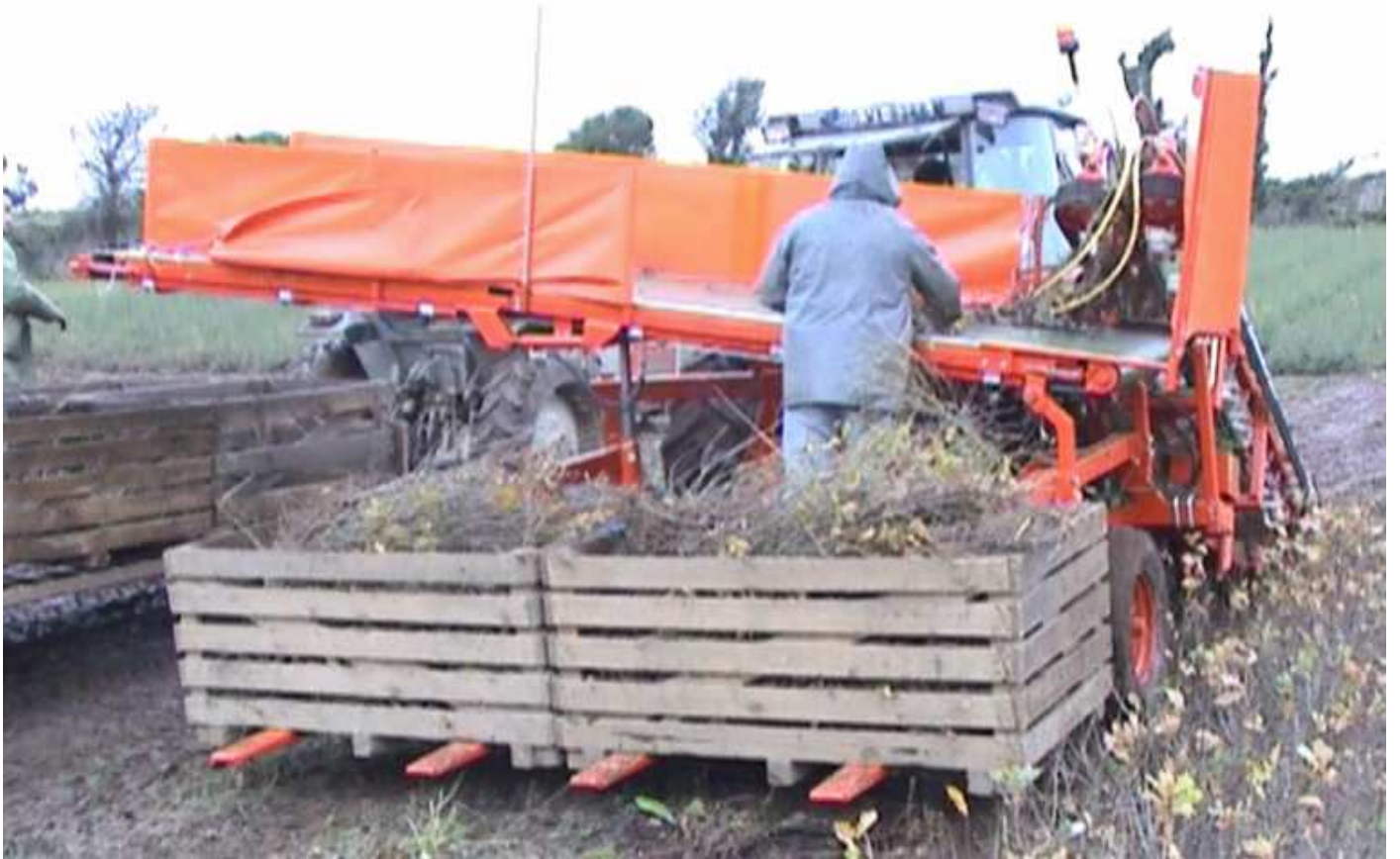
custom made machine to load directly on a trailer
