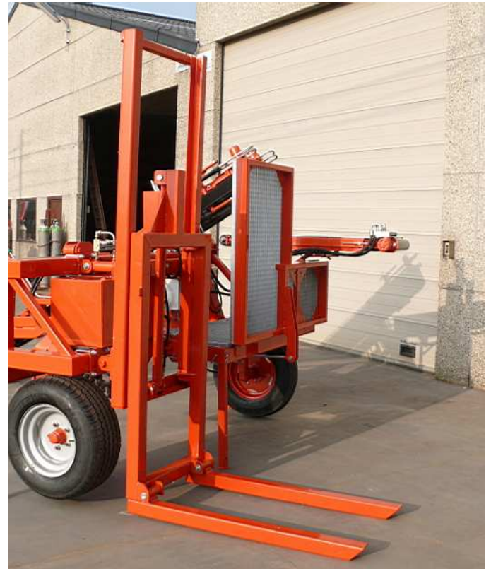
ZLX, platform folds upwards by hydraulics
