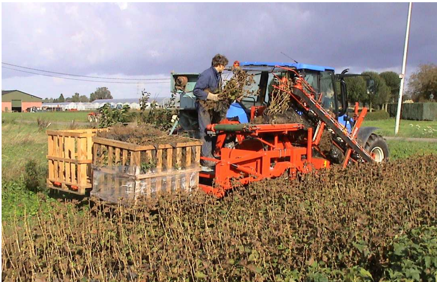
AL + RASSPE, with extra big platform and enough space for a Rasspe tying machine. Elevator on the back with 2 or 4 forks.
