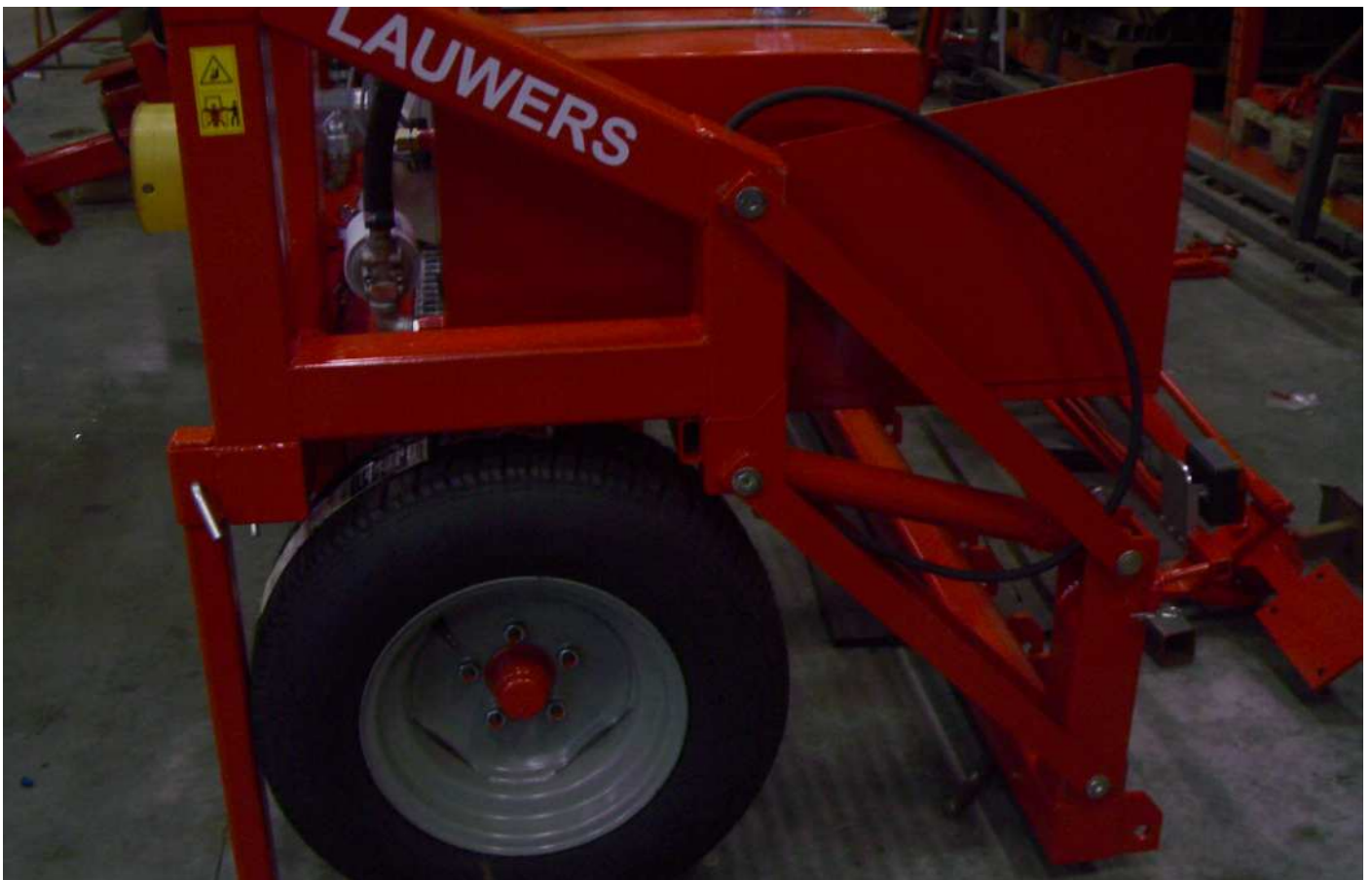
ALC, short frame = weight of machine and pallet close to the tractor. Platform 1,1 m long.
